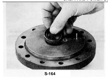
The steering gear bearing cap and high-pressure oil seal are serviced in the same manner as the fixed miter gear assembly. Refer to the fixed miter section of this manual for complete details..
