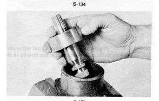
Carefully tap or press miter shaft out of the bearing.
