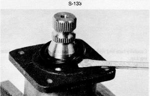
Remove seal from miter cover.
