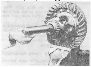
B. Insert checking tool (made from splined axle shaft end) into differential nest. Allow splines of tool to engage with spline of one side gear only.
