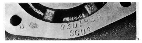
A number is cast into the steering gear housing and identifies the basic family to which the steering gear belongs. 392-S would indicate a :392 short series steering gear. See series 4 and series 5 example below.
